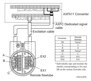
Figure 4.4.5 Wiring Diagram
